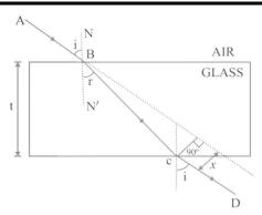
Lateral shift  $x = \frac{t \sin(i-r)}{\cos r}$ ; t = thickness of slab
