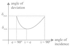
• There is one and only one angle of incidence for which the angle of deviation is minimum. When  $\delta = \delta_{min}$  then i = i' and r = r', the ray passes symmetrically about the prism,
