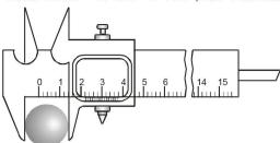
**Ex.** A vernier scale has 10 parts, which are equal to 9 parts of main scale having each path equal to 1 mm then least count = 1 mm  $-\frac{9}{10}$  mm = 0.1 mm [ $\because$  9 MSD = 10 VSD]
