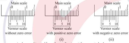
The zero error is always subtracted from the reading to get the corrected value. If the zero error is positive, its value is calculated as we take any normal reading. Negative zero error  $= -[Total\ no.\ of\ vsd-vsd\ coinciding] \times L.C.$
