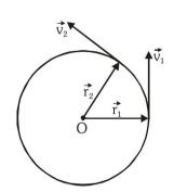
due to centripetal acceleration, the velocity of the particle keeps on changing the direction i.e. the particle is accelerated.
