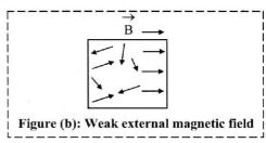
A complete alignment is prevented due to thermal vibration. The specimen has acquired a net dipole moment  $\vec{M}$ .
