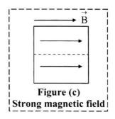
When the external applied magnetic field is strong as shown in figure (c), the dipole moments of non-aligned domains abruptly rotate in the direction of the applied field. Removal of external field does not set the domain boundaries back to their original position, and the material gets the magnetic property permanently.
