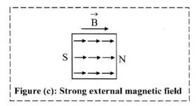
The net magnetic dipole moment is parallel to  $\vec{B}$ . Hence the specimen shows a tendency to move from weaker field to stronger field.
