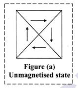
In the absence of any external magnetic field, the different domains are oriented at random -so that the magnetic fields of the domains cancel each other and does not show any magnetic (effect) properties, as shown in figure (a).
