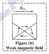
When the external applied magnetic field is weak, the individual atomic magnets tend to align their dipole moments parallel to the direction of the field, as shown in figure (b). The domain wall shifts in the direction of applied field. With the removal of the external magnetic field, the boundaries return to their original positions and the material loses its magnetism.
