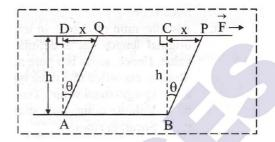
ii. In the figure, base of the block AB is fixed. A tangential force 'F' is applied to the upper surface so that lateral displacement of the face is 'x'.
