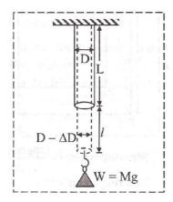
iv. Longitudinal strain in the wire is given by,
