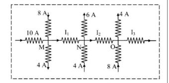
**6.** In the circuit shown below calculate the value of the current 1.
