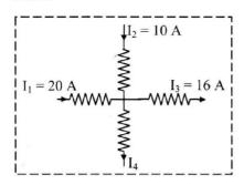
5. In the circuit shown below, calculate the value of currents  $I_1$ ,  $I_2$  and  $I_3$ .
