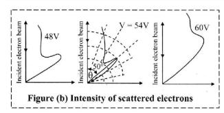
The size of the bump becomes maximum, when accelerating voltage is 54 V.
