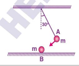
Ans. In an elastic collision when the ball A hits the ball B which is stationary, the ball B acquires the velocity of the ball A while the ball A comes to rest immediately after the collision. There is a transfer of momentum to the moving body from the stationary body. Thus, the ball A comes to rest after collision and ball B moves with the velocity of ball A.
